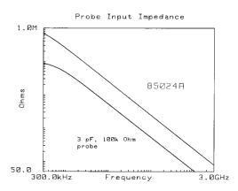
Probe with less error due to higher input impedance. For example, in a 50  $\Omega$  system at 500 MHz, the 85024A presents 455  $\Omega$  which produces a 10% signal loss from loading effects, while a 3 pF, 100 k $\Omega$  probe presents 106  $\Omega$  causing a 32% signal loss.
